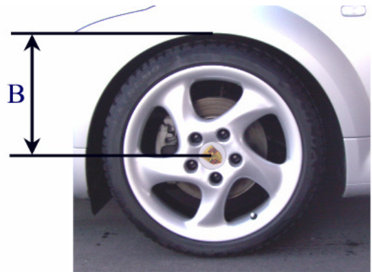
Measurement B Wheel hub center wheel arch
