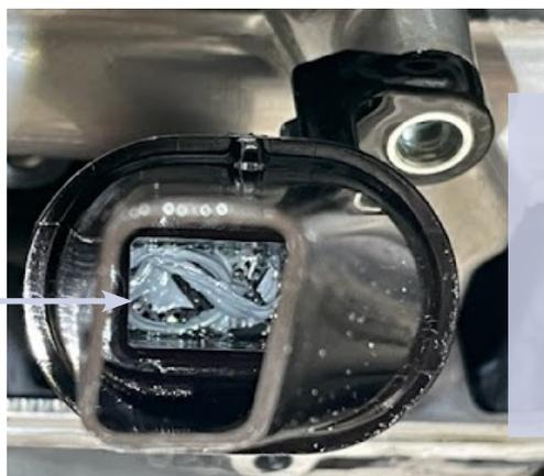
In these pictures you can see how **the excess silicone** in the crankcase has come loose and has been sucked into the lubrication system, clogging the pre-filter.
