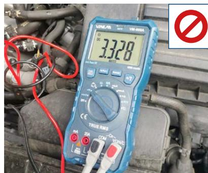
If you measure a voltage of approximately 3.3 V, the glow plug is not compatible with this vehicle.
