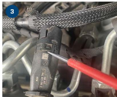
Remove the protective cap at the front with a small screwdriver.
