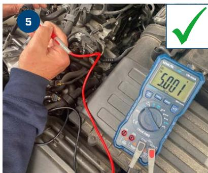
The displayed voltage must be in the range between 4.8 and 5.2 V.
