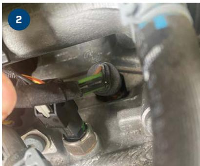
You can identify the pressure sensor glow plug by the fact that a 4-pin connector is attached to it. Remove the connector carefully.
