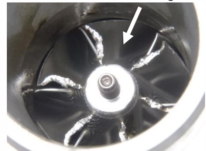
Rotor shaft nut is missing !
