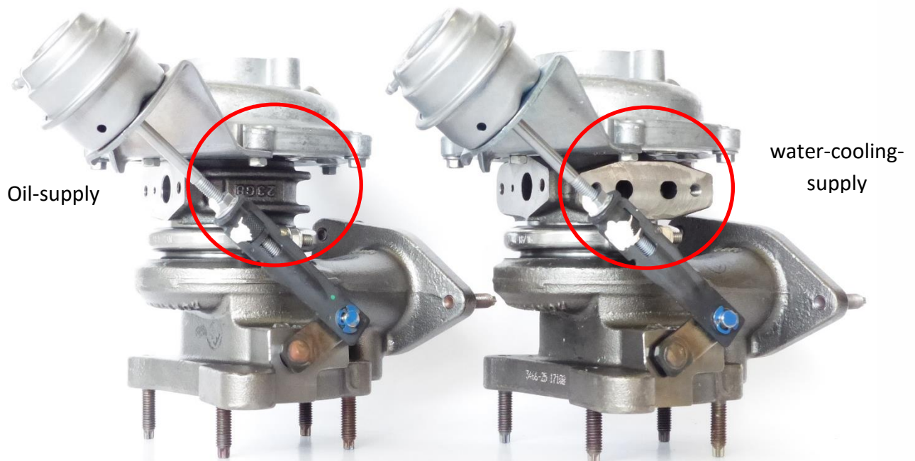
T916692 without water-cooled bearing housing
