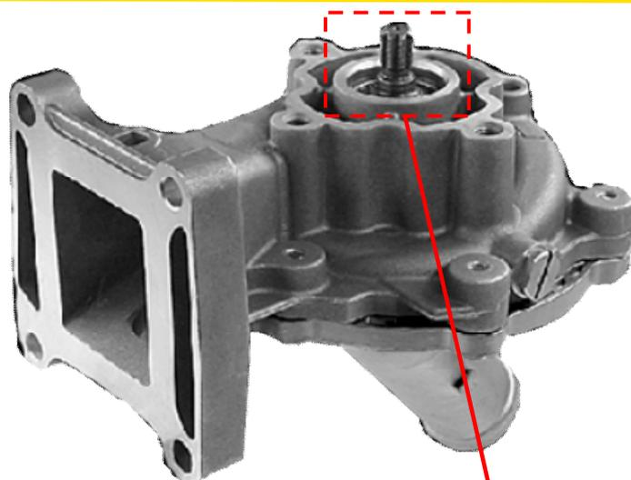
During the assembly of the pump, the shaft spline must be coated with a suitable high performance-temperature fat paste like Molykote M-77 assembly paste or similar!
