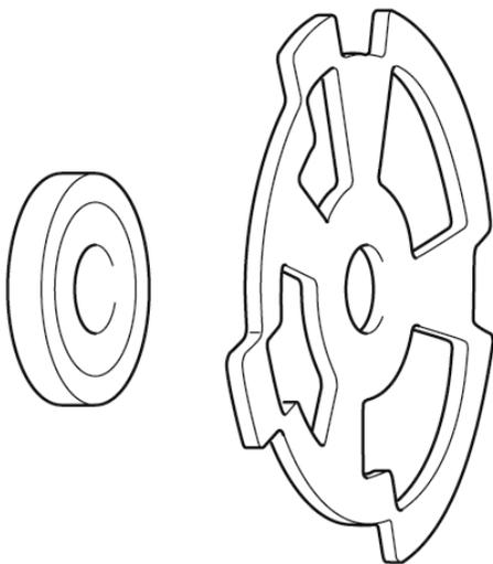
Fig. 1: Encoder wheel with pressed-out spacer ring
