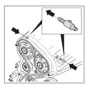
In order to ensure that the new camshaft phasing units operate correctly, the control valves included in the INA Engine KIT must be used.
