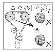
The control valve filters are clogged due to dirt and abrasion. As a result, the camshaft phasing units are not supplied with sufficient engine oil and are irreparably damaged. This damage is evident in the form of significant noise generation and/or oil leakage.
