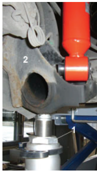
Fig. 7: 1 Wagenheber / Jack / Cric / Gato elevador 2 Radträger / Wheel carrier / Support de roue / Rótula
