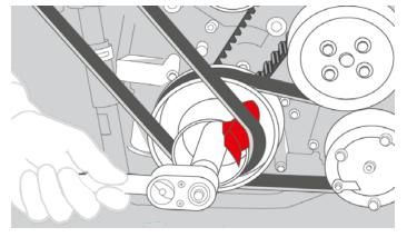
2.Use a ratchet to turn the crankshaft in a clockwise direction. The belt can then be lifted off the pulley, and slid off the tool.
