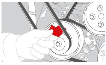
1. Position the removal tool between the pulley and the belts, as shown.
