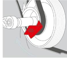
2. Use a ratchet to turn the crankshaft in a clockwise direction in order to install the elastic belt.
