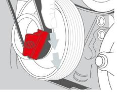
1.Place the installation tool over the crankshaft pulley and pass the belt over the leading edge of the tool.
