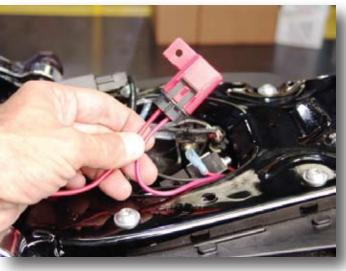
6. The system is equipped with a relay, refer to the included schematic for a wiring diagram. Locate the fuse assembly close to the battery. Connect the ring terminaled end of the fuse harness to battery positive (+). Reconnect the battery cables, tighten to 60-96 in-lbs. (6.8-10.9 Nm).
