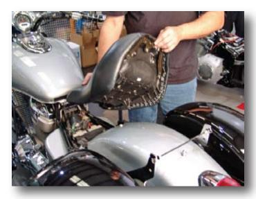
7. Once the system is operational, use a soap and water solution to check for any leaks. Reinstall the side cover and seat, check to ensure the seat is securely locked in the frame
