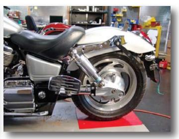
8. Make sure that there is adequate clearance between the rear tire and fender being sure to check both the sides and the top. Roll the bike backwards and forwards with no air in the system feeling for any friction.
