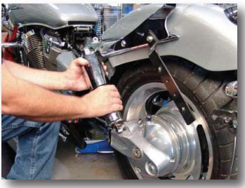
4. Carefully remove factory shock absorbers from the rear suspension.
