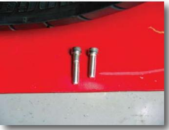
2. Supplied with the kit are 6 new mounting bolts, the 2-longer bolts are to be used on the top mount of the VTX®. The 4-shorter bolts are for the lower VTX® mounts and all 4 of the Rocket® III mounts.
