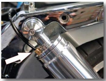
4. Route the 4mm line from the manifold to the shocks and connect to each using the 4mm VOSS® fittings.
