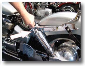
2. Loosen and remove the upper shock mounting hardware.
