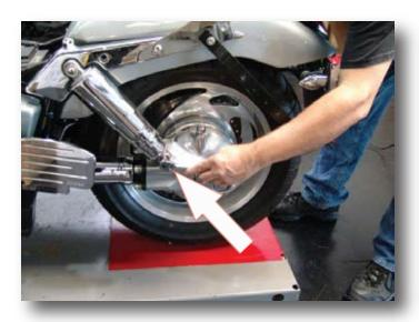
3. Loosen and remove the lower shock mounting hardware.
