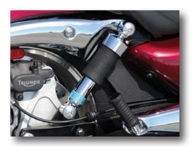
3. Mount the new shocks one at a time starting with the lower mount first, then adjust the height of the bike to align the upper mount. Tighten all shock mounting hardware to 25 ft-lbs. (34 Nm).
