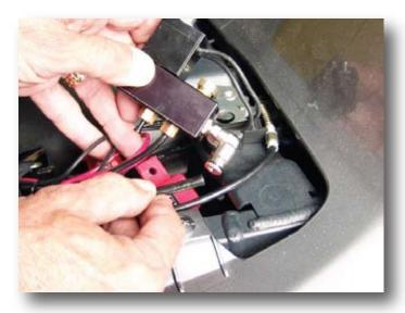
3. Locate a suitable location to mount the manifold. Connect the ¼" line, leading from the compressor, to the valve block via the "push to connect" fitting. Supplied with the kit is a speed reducing muffler than can be used to slow the speed of the drop. If used it is to be threaded into the open port opposite of the elbow.
