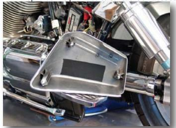
1. A preferred mounting location is under the bike's left side cover. Use the Velcro® strip supplied in the kit and attach one side to the side cover and the other to the compressor.
