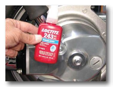
1. Before final assembly, apply 2-3 drops of Loctite® 243 (Blue), to the threads of all shock mounting hardware.
