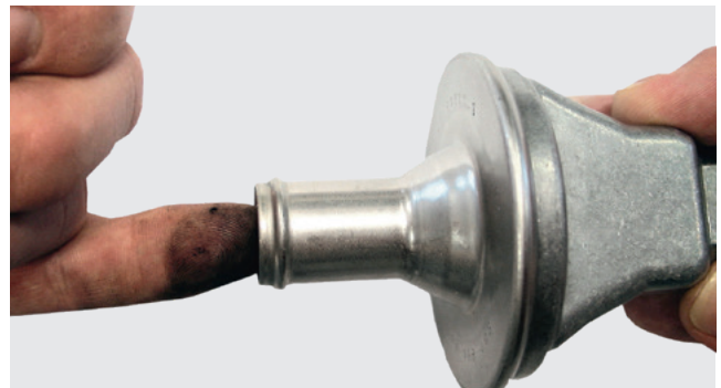
Fig. 1: Simple inspection of the non-return valve
