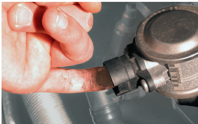
Quick inspection of the secondary air valve in the BMW 520i (highlighted)
