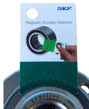
ABS magnetic impulse ring in bad condition. The magnetic sensor ring is damaged, some segments are no longer separated from each other and thus can no longer indicate an even speed signal.
