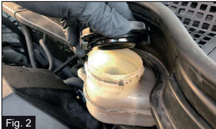
Remove the cover from the expansion tank
