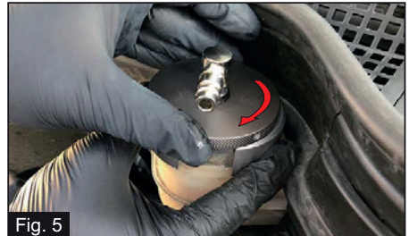
Push the locking arms back together as far as they will go and tighten the lid by turning it.
