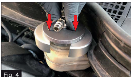
Insert the adaptor cover and push it down as far as it will go
