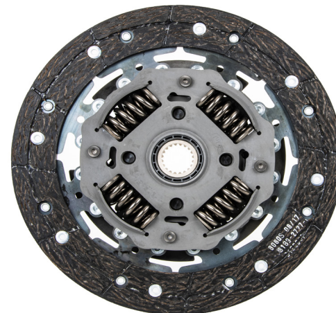
Fig. 2: LuK clutch disc with centrifugal pendulum-type absorbers (drive side)
