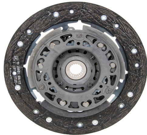
Fig. 1: LuK clutch disc with centrifugal pendulum-type absorbers (flywheel side)
