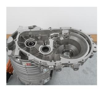
• Remove the shaft oil seal of the rotor shaft
