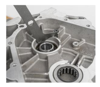
• Press in new rotor shaft oil seal to previous installation depth
