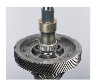
• Press a new tapered roller bearing on the motor side of the differential
