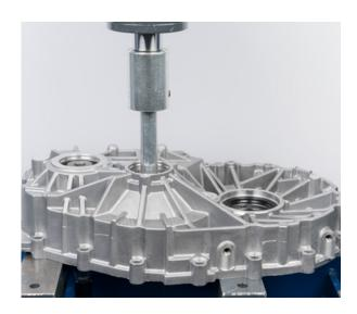
• Press out the input shaft from gearbox housing
