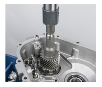
Press the output shaft into the gearbox housing
