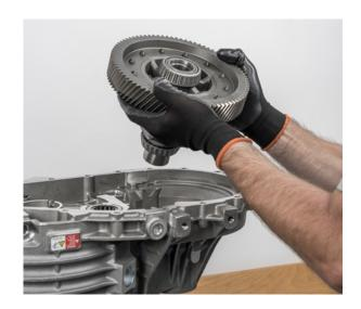
• Remove again the outer bearing race on the motor side of the differential gear
