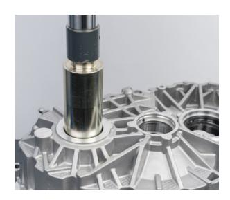
• Remove the drive shaft flange oil seal from the gearbox side
