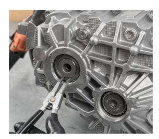
• Remove the output shaft bolt
