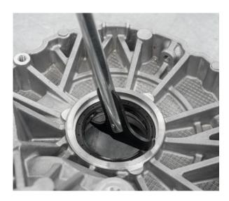
• Remove the bearing outer race from the gearbox side using a suitable internal extractor
