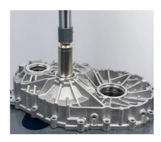
• Press out the input shaft ball bearing from the gearbox housing
