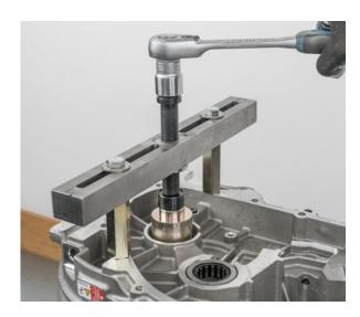
• Remove the motor side bearing of output shaft with suitable internal extractor
