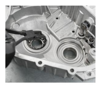
• Press out the output shaft angular contact ball bearing from the gearbox housing
