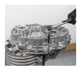
Mount the dial gauge as shown and ensure that the measuring tip is pretensioned
