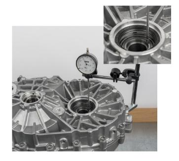
Press the differential gear on the opposite side upwards by hand until it stops and read the measured value
