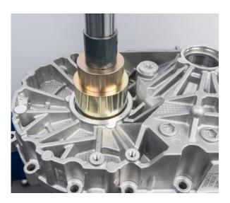
• Press new ball bearing of the input shaft into the gearbox housing
