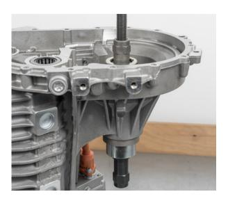
Remove the bearing inner race on the gearbox side of the output shaft using a suitable inner race puller
