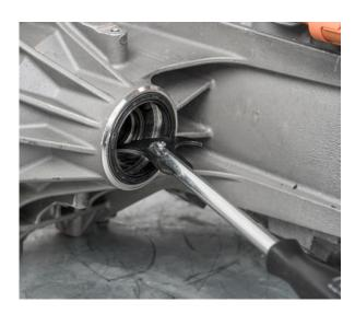
• Remove both sealing caps using a suitable tool, e.g. Gedore Automotive KL-0369-59
