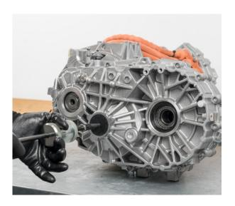
• Remove the snap ring from the input shaft
