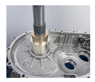
• Press the new oil seal on the gearbox side of the differential into the gearbox housing
