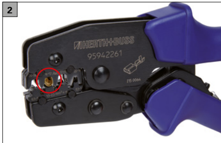
2 Insert terminal into the profile. Close the tool slightly until the terminal is hold.
