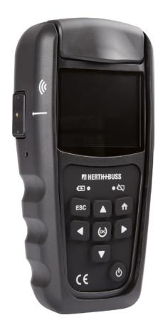
The AirGuard is a programming and diagnostic device. It allows work to be carried out directly on the vehicle whilst offline. The vehicle database, with a coverage of 80-90%, is stored in the device itself. Updates are available free of charge from our website. The AirGuard is able to read out all sensor types found on the market. Then, it is able to automatically or manually duplicate the read data to the Herth+Buss wheel sensors. Programming a new sensor ID is also possible, as well
